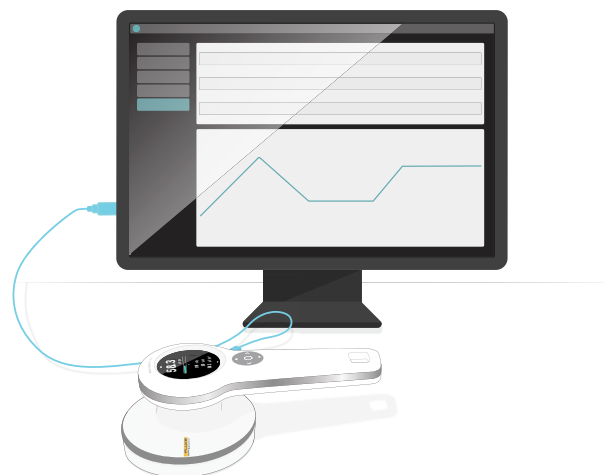
Figure 10. Connect instrument to RaySafe View.
