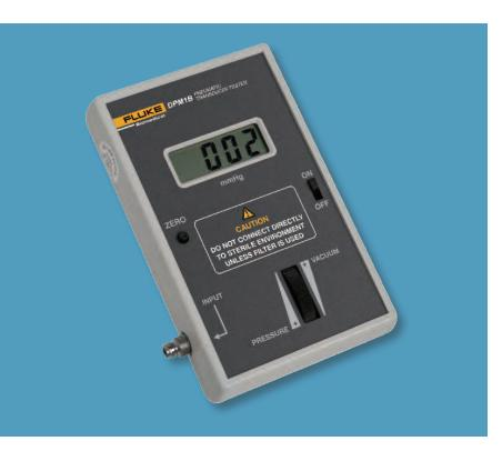
The DPM1B pneumatic transducer tester is designed to measure the positive and negative pressures of medical devices in either liquid or gaseous form, and to generate pressure within the  $\pm$  300 mmHg range to assist in repair and quality control.
