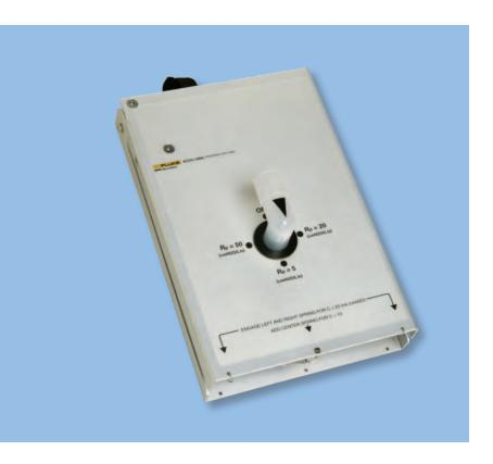
The ACCU LUNG Precision Test Lung is a lung simulator that presents a specific load comprised of user-selectable compliance and resistance for the purpose of evaluating ventilator performance according to clinical expectation and manufacturers' specification. It is a portable unit that can be hung from a cart, the ventilator itself, or hand-held, thus presenting a zero footprint.
